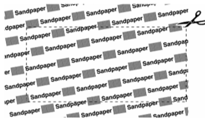
Figure 6.3.3.7-2. Barcode placement on random-wrapped item
